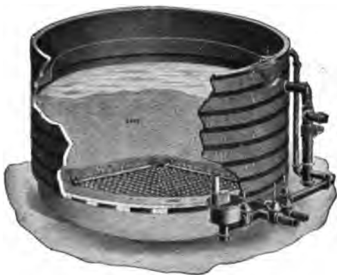
FIG. 44.—Gravity type of mechanical filter.
